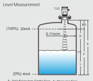
E : Total Range from X'mitter Face, F : Measuring Span, BD : Blanking Distance, D : Distance, L : Level ( E - D )
